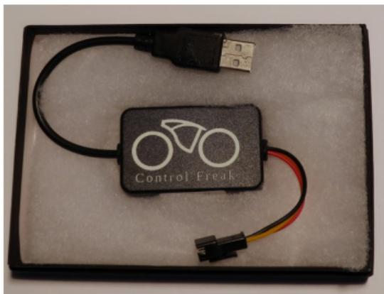
Multiple controllers can be synchronized together so that they respond as one to power up/down, or changes in Effects, Color, and Intensity. This is perfect for the typical bike installation, where electrically separate LED, controller, and power-packs are installed on each wheel, and the frame. With the Control Freak system, a Model LBCF-L, which has a push button, can be installed on the frame, and used to control Model LBCF-F controllers on the wheels.
